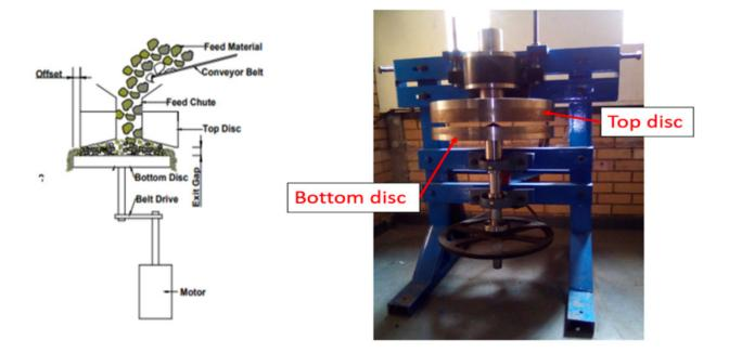
Working diagram for the rotary offset crusher (left) and photograph showing the discs (right)
