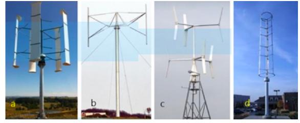
(a) High solidity Giromill; (b) H-rotor; (c) Two-stage Giromill; (d) High aspect ratio Darrieus turbine.
