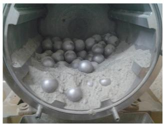
A ball mill grinder with large balls and large lifters on the inner wall.
