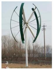
Curved blade assembled on turbine
