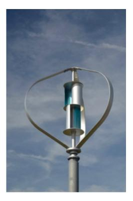
Whereas the Savonius-Vanes are drag-driven, the Darrieus-Blades will experience a lifting force when wind is blowing across the turbine. Since a pure Darrieus Wind Turbine is (mostly) not able to start without an initial net rotational force, the Savonius-Vanes are added to make the turbine self-starting. This system is omnidirectional and does not need special yaw
