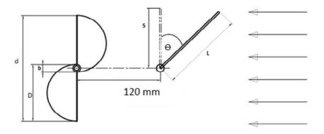
Schematic illustration of the turbine and flat plate obstacle upstream of the returning blade (Putri et al, 2019)
