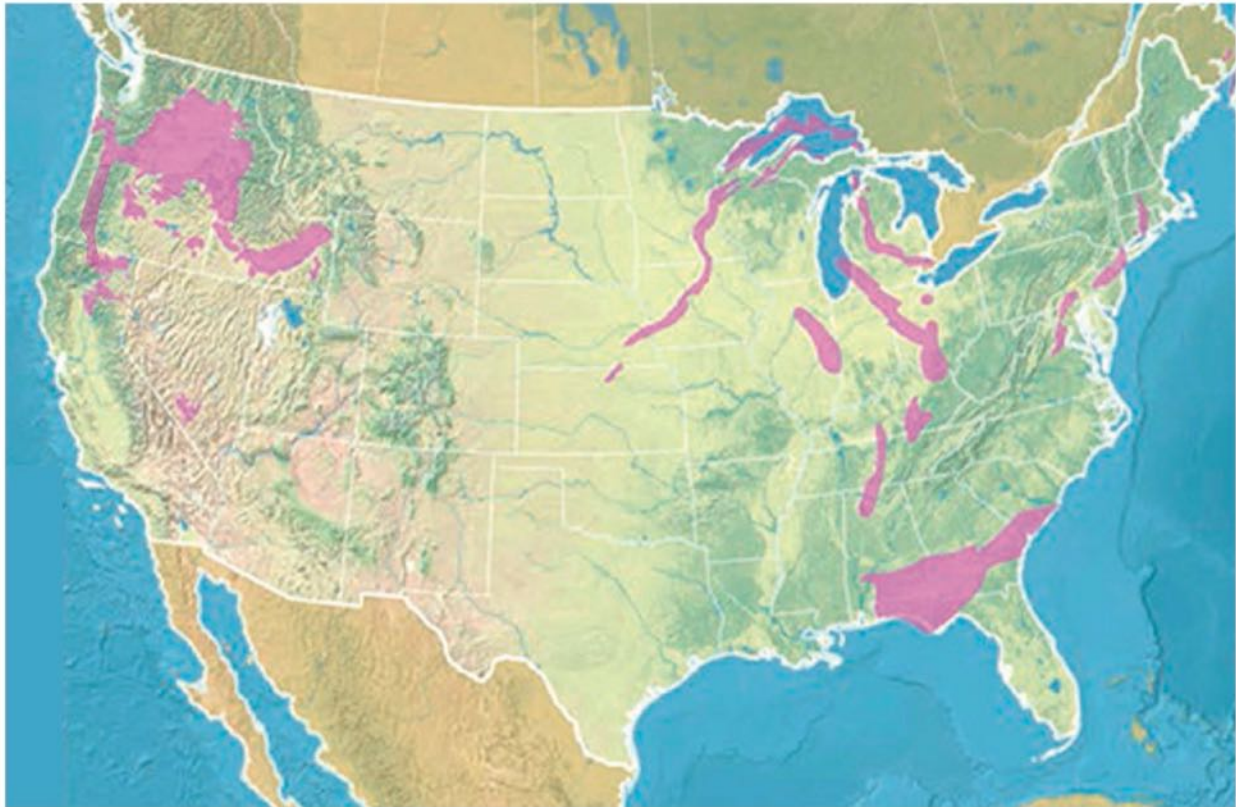
Credit: US Department of Energy/National Academies of Sciences, Engineering, and Medicine. Map of basalt formations (red) at and near the surface of the US that would be suitable for CO 2 sequestration.
