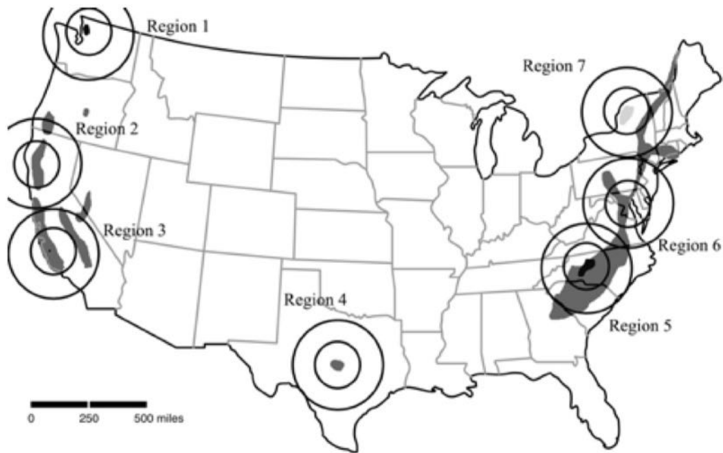
Ultramafic Mineralization Carbonation sites. Regions 1 and 5 contain olivine; regions 2-4 contain lizardite serpentine; region 6 contains antigorite serpentine; and region 7 contains wollastonite. 5 = Asheville Mining District
