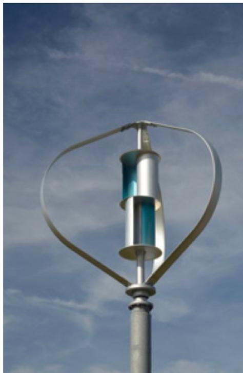
Whereas the Savonius-Vanes are drag-driven, the Darrieus-Blades will experience a lifting force when wind is blowing across the turbine. Since a pure Darrieus Wind Turbine is (mostly) not able to start without an initial net rotational force, the Savonius-Vanes are added to make the turbine self-starting. This system is omnidirectional and does not need special yaw
