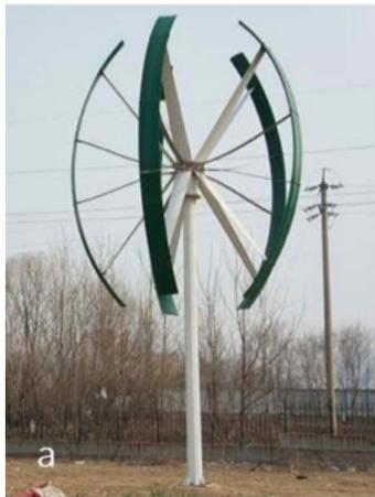
Curved blade assembled on turbine
