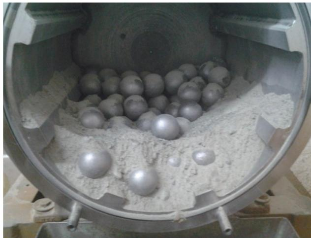
A ball mill grinder with large balls and large lifters on the inner wall.
