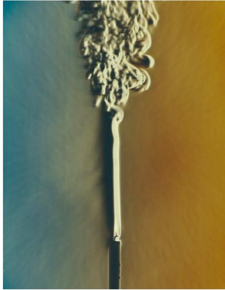
The plume from this candle flame goes from laminar to turbulent. The Reynolds number can be used to predict where this transition will take place.
